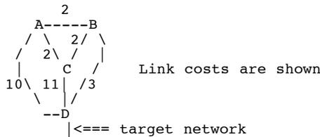
If the link from B to D goes down, show what the sequence of distances/next hops is for each router to the target network, assuming routers send updates at the same time, using...
