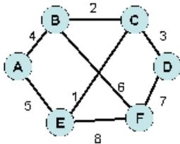
14. For the following network, what is the distance and next hop from each router to the target network?
