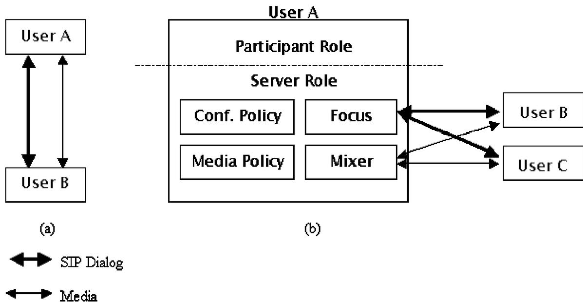
Figure 3.3 - Endpoint Server ([ID FRAMEWORK-00])
