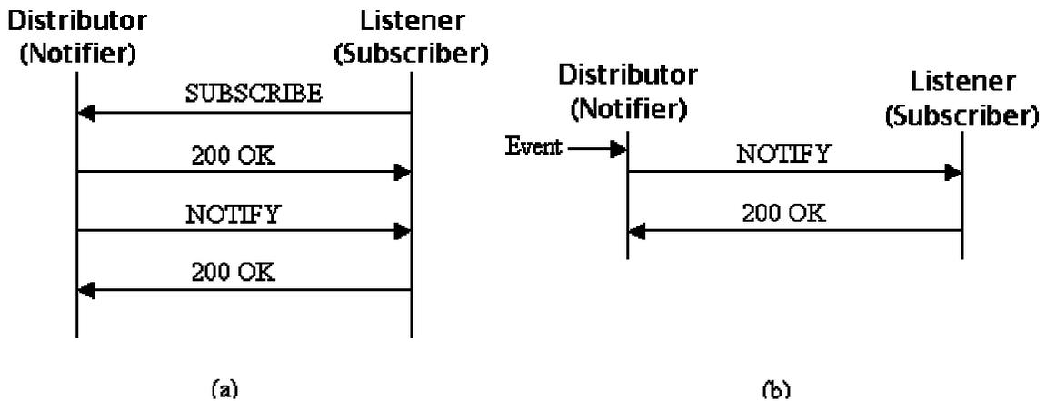
**Figure 2.3** - SIP Events Mechanism (a)REGISTER and (b)NOTIFY
