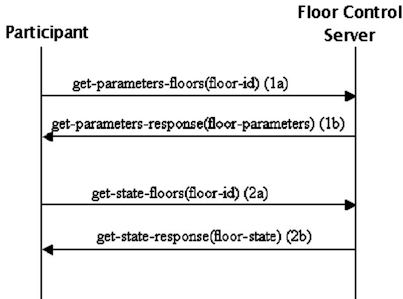
Figure 4.35 - Get Floor Parameters and State Procedures
